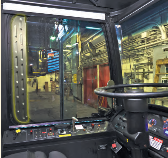
A Bus Operator window with louvers to protect the Operator from riders outside is being tested on a bus operating out of the Manhattanville Bus Depot.
