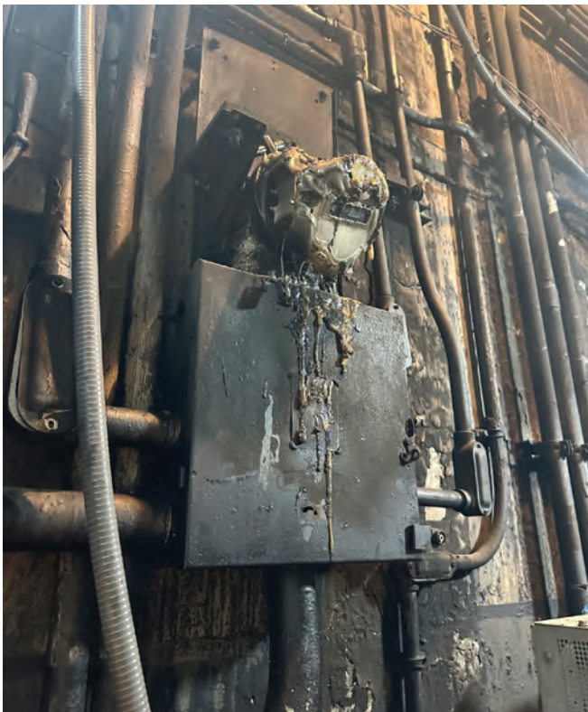
The heat of the fire and explosion baked components
